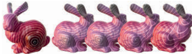
Figure 11. A source on the front of the Stanford Bunny results in nonsmooth cusps on the opposite side. By running heat flow for progressively longer durations t , we obtain smoothed approximations of geodesic distance (right).
