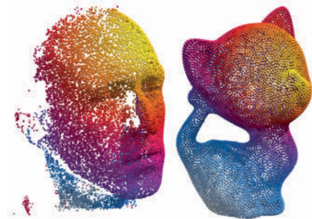
Figure 10. The heat method can be applied directly to scattered point clouds. Left: face scan with holes and noise. Right: kitten surface with connectivity removed. Yellow points are close to the source.
