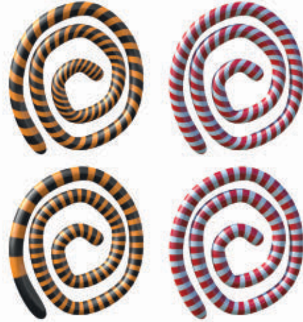
Figure 8. Left: Varadhan’s formula. Right: the heat method. Even for very small values of t , simply applying Varadhan’s formula does not provide an accurate approximation of geodesic distance (top left); for large values of t spacing becomes even more uneven (bottom left). Normalizing the gradient results in a more accurate solution, as indicated by evenly spaced isolines (top right), and is also valuable when constructing a smoothed distance function (bottom right).
