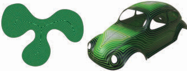
Figure 7. Distance to the boundary on a region in the plane (left) or a surface in space (right) is achieved by simply placing heat along the boundary curve.
